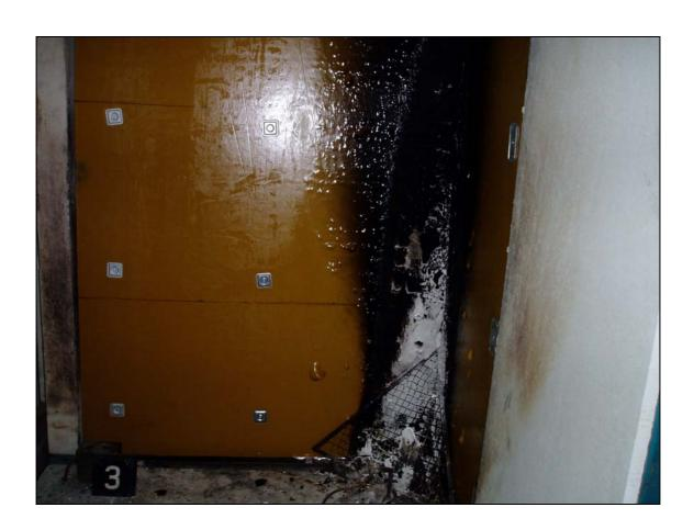
PHOTO N°10: Sample n°3 – Product status upon completion of the test.
