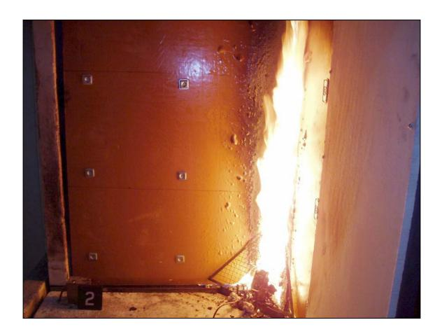
**PHOTO N°7:** Sample  $n^{o}2$  – Flame attack approx. 10 minutes after the start of the test.
