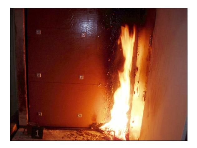
**PHOTO N°5:** Sample  $n^0\mathbf{1}$  – Flame attack approx. 10 minutes after the start of the test.
