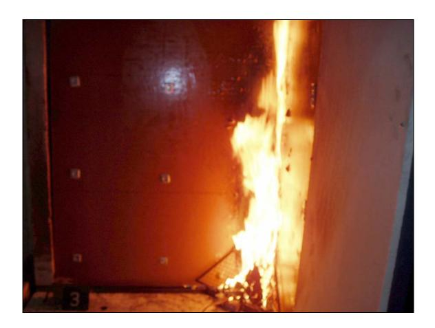
**PHOTO N°9:** Sample n°3 – Flame attack approx. 10 minutes after the start of the test.
