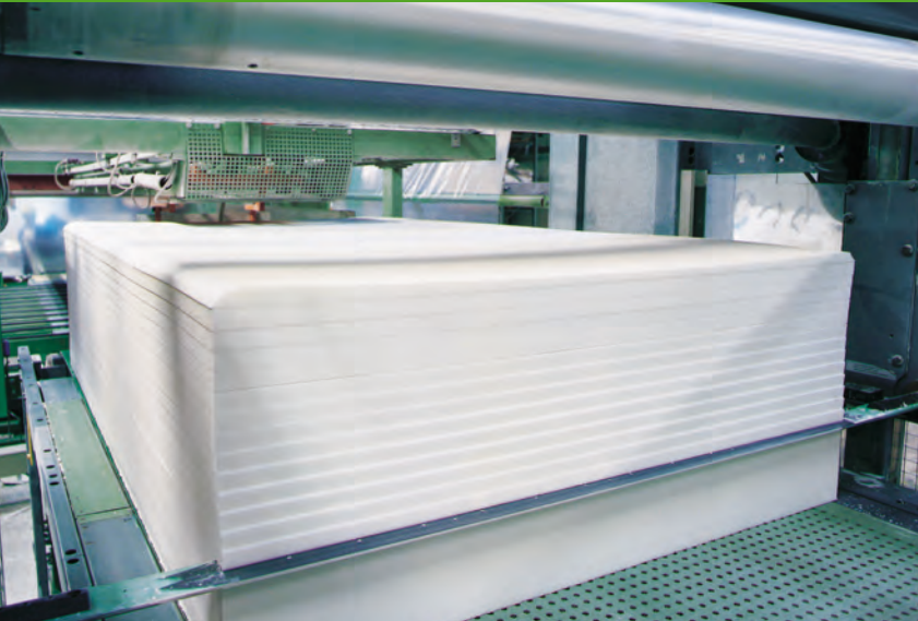
Cutting of Basotect® panels
